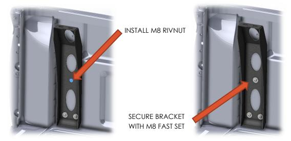
✓ Place the FRT fitment bracket in position and secure with  $2 \times M8$  body washers,  $2 \times M8$  spring washers and  $2 \times M8 \times 25$  bolts at the bottom. Repeat on right hand side.
