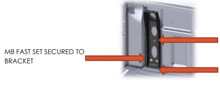
USE INDICATED HOLE AS DRILL JIG FOR Ø11mm HOLE SHOULD THE LOAD BIN BE PRE-FITTED WITH A LOAD MAT, THE LOAD MAT WILL HAVE TO BE TRIMMED TO SUIT THE FITMENT BRACKET.
