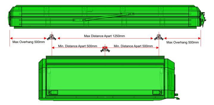
On a ute/pickup, due to the difference in flex between the cab and the tray/canopy, you must not fix the tent across the two, as this will result in damage to the tent and also your vehicle.
